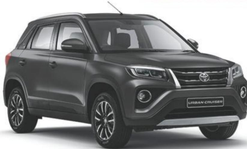
Buyers can choose 5-speed manual or 4-speed automatic transmission, driving the front wheels.
